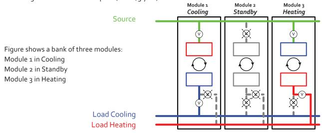
\*Simplified single line water circuit shown; V=motorized isolation and control valve
