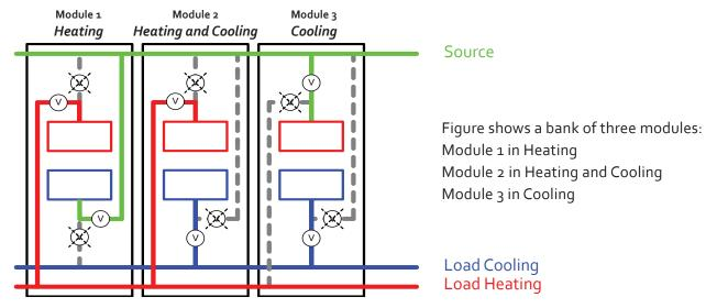
\*Simplified single line water circuit shown; V=motorized isolation and control valve
